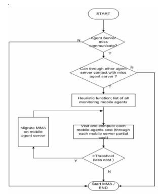
Figure 5 MMA self-relocation algorithms
